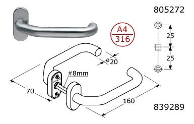
door lever handles stainless steel 316/A4 satin polished also for narrow profile doors, total highness 70mm with stainless steel 316/A4 handles ø20x160mm ### nice finish & for all kind of situations.
