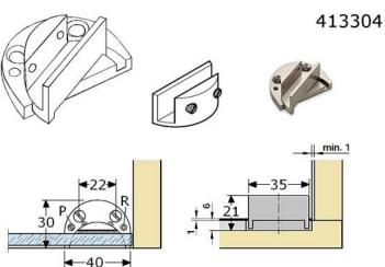
pivot glass door hinges, highness 21mm brass satin nickel plated for glass thickness 4-8mm, maximum loading 4 Kg (for 2 Pcs: maximum door width 450mm) no hole in glass, pre-drilling not required mounting/pinching with 2 nice screws M4 for inset/recessed showcase glass doors turning in special groove, not selfclosing after mounting: place safety stopper screw P or R bottom mounting with 2 countersunked screwholes with distance plates rounded bottom hole necessary in boxes of 12 Pcs.
