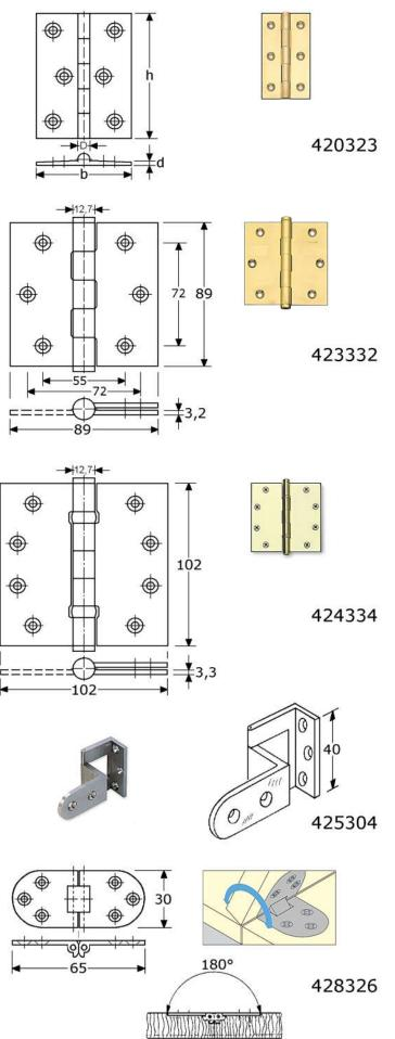
for table top hinges for 180° opening fully flat out of stainless steel, see page GY-382b (group 03) butt hinges with fixed brass pin brass profile, polished flat surface mounting, thickness 1,5-1,8mm 5-knuckles ø4,5mm, without tips with 6 countersunked screwholes
