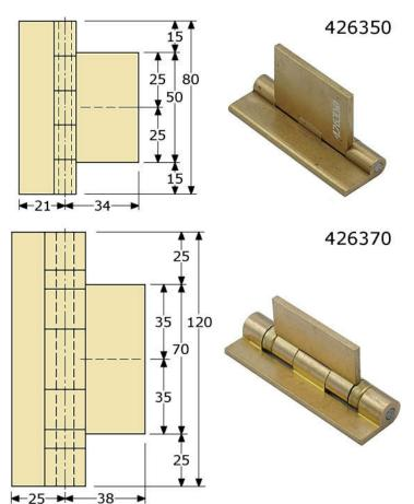
solid profile hinges 80/50x55x3,5mm brass profile unpolished, 5-knuckles ø10mm without holes, middle profile highness 50mm cranked 6,5mm, without bearing with fixed stainless steel 430 pin ø5mm total widthness 21+34=55mm in boxes of 10 Pcs. (delivery on request)
