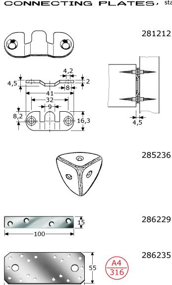
connecting plate 41x16,3mm stainless steel 304/A2 satin thickness 2mm ### two pieces together = thickness 4,5mm ### with 2 countersunked screwholes (3,5mm) in boxes of 100 Pcs. and 500 Pcs.
