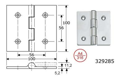
butt hinges with fixed stainless steel pin stainless steel 316/A4/1.4401 mirror polished flat surface mounting, 4-knuckles ø11,2mm solid casting, no bearing widthness 100mm (50+50mm) with 4 countersunked screwholes (5mm/M5)
