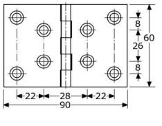
rolled back flap hinges with fixed riveted (SS) pin stainless steel 304/A2/1.4301, flat surface mounting with 8 countersunked screwholes (4mm/M4)
