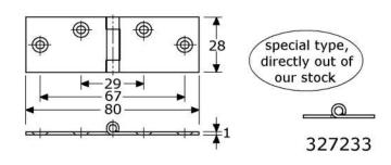
rolled back flap hinges with fixed riveted (SS) pin stainless steel 304/A2/1.4301, 3-knuckles flat surface mounting; special, but stock article !!! with 2+2 countersunked screwholes (3mm/M3)
