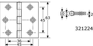
rolled hinges with fixed riveted stainless steel pin stainless steel 304/A2/1.4301, swaged with 6 countersunked screwholes (4mm/M4)
