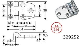
offset hinges with fixed stainless steel pin stainless steel 316/A4/1.4401 mirror polished solid casting, 4-knuckles with 9,5mm offset widthness 54mm (17+37mm) with 5 countersunked screwholes (4,8mm/M5)
