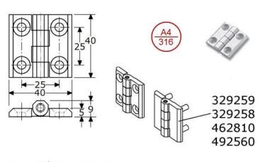
butt hinges with fixed SS-304 pin ø4mm stainless steel 316/1.4571 satin polished flat surface mounting, 4-knuckles solid casting, smooth border with 4 countersunked screwholes (5mm/M5)
