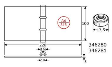
rolled hinges with LOOSE stainless steel pin ø10mm stainless steel 316/A4/1.4401 satin polished flat surface mounting, 3-knuckles ø16mm pin & buttom tip out of stainless steel 316/A4 with each 2 ball bearings stainless steel ø17,5mm (outside & inside SS-304/A2, balls SS-420 harded) without screwholes
