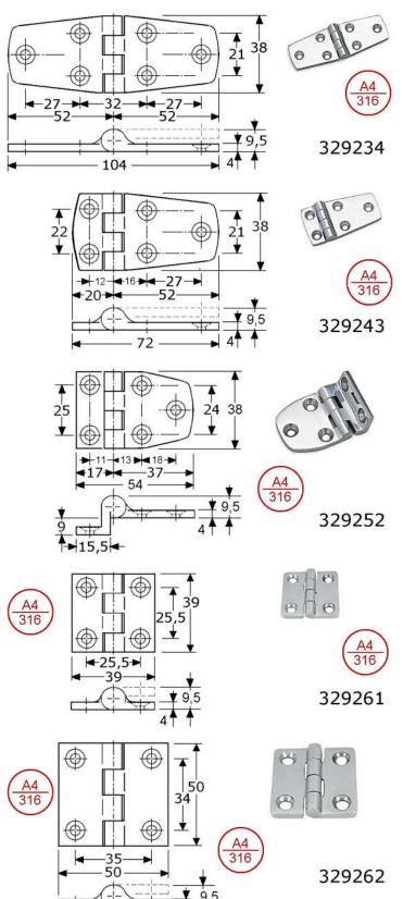
strap hinges with fixed stainless steel pin stainless steel 316/A4/1.4401 mirror polished solid casting, flat surface mounting, 4-knuckles widthness 104mm (52+52mm)
