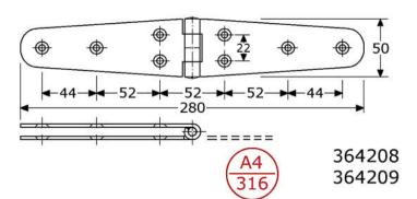
strap hinges with fixed stainless steel pin stainless steel 316/A4/1.4401 flat surface mounting, rolled, tapped rounded leaves with fixed riveted stainless steel pin, no bearing widthness 280mm (140+140mm), 3-knuckles with 8 countersunked screwholes (6mm/M6)
