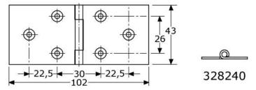
rolled back flap hinges with fixed riveted (SS) pin stainless steel 304/A2/1.4301, flat surface mounting with 6 countersunked screwholes (4mm/M4)
