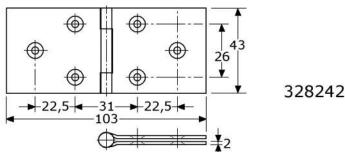
rolled hinges with fixed riveted stainless steel pin stainless steel 304/A2/1.4301, swaged with 6 countersunked screwholes (4mm/M4)
