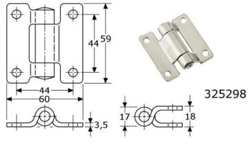
rolled hinges with fixed riveted stainless steel pin stainless steel 304/A2/1.4301 flat surface mounting, rolled, rounded with 4 round holes ø6,5mm
