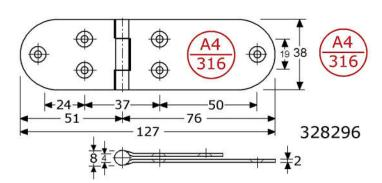
rolled hinges with fixed riveted (SS-316/A4) pin stainless steel 316/A4/1.4401 satin polished swaged rolled, rounded, 3-knuckles widthness 127mm (51+76mm) with 6 countersunked screwholes (3,5mm/M4)
