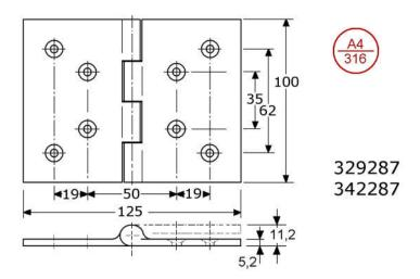
butt hinges with fixed stainless steel pin stainless steel 316/A4/1.4401 mirror polished flat surface mounting, 4-knuckles ø11,2mm solid casting, no bearing widthness 125mm (62½ + 62½mm) with 8 countersunked screwholes (5mm/M5)
