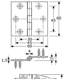
hinges with fixed riveted (SS) pin stainless steel 304/A2/1.4301, 3-knuckles contra mounted with 5,5mm offset ### special type & directly out of our stock ### with 6 countersunked screwholes (3,5mm/M4)
