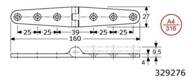
strap hinges with fixed stainless steel pin stainless steel 316/A4/1.4401 mirror polished flat surface mounting, 3-knuckles ø9,5mm solid casting, no bearing widthness 160mm (80+80mm) with 6 countersunked screwholes (5mm/M5)
