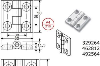
butt hinges with fixed SS-304 pin ø6mm stainless steel 316/1.4571 satin polished flat surface mounting, 4-knuckles solid casting (back not flat), smooth border with 4 countersunked screwholes (6mm/M6)
