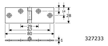
rolled back flap hinges with fixed riveted (SS) pin stainless steel 304/A2/1.4301, 3-knuckles flat surface mounting; special, but stock article !!! ### special type & directly out of our stock ### with 2+2 countersunked screwholes (3mm/M3)
