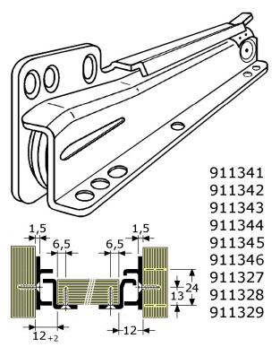
single extension drawer slide (2-parts) steel white coated or steel cream coated (RAL-9001) single extension 75% space required 12mm, for bottom mounting with (per pair) 4 rollers ø22mm non-return groove in the front of the cabinet profile for keeping the drawer in closed position
