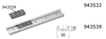
guide rails 200mm with widthness 30mm aluminium anodised profile, highness 10mm highness 10mm, max. loading 15 Kg/Pr (vertical) (delivery on request; also possible 400/800mm)
