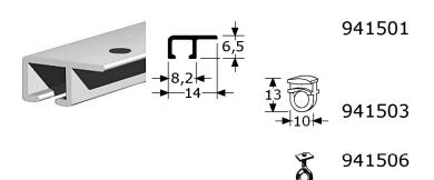
curtain rail 14x6,5mm aluminium profile small type, for yacht interior use in boxes of 100 Mtr (20 Pcs. of 5 meter)
