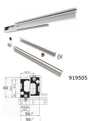
heavy duty drawer slides aluminium alloy profile single extension 70% space required 56mm, highness required 60mm
