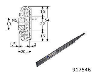
precision ball bearing slides aluminium alloy profile full extension slide, extension lenghts 100% space require 20,1mm, highness 54mm, side mounting with steel ball bearing can not be disconnected, non handed load capacity based on normal vertical (drawer) use the outer rail: with double holes for 5mm the inner rail: with single tapped holes M6 sales by pair (but left & right are the same) delivery on request (A)
