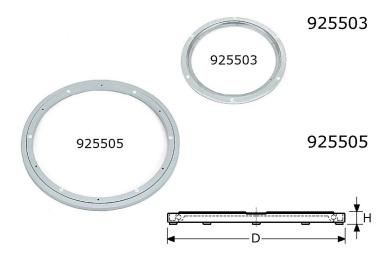
rotary ring/swivel, outside ø326mm aluminium alloy/profile, highness 16mm with big steel ball bearing, for 60 Kg rotary 360° without stop (not demontable) with white rubber stoppers prevent slipping top ring has 6 countersunked holes to fix on table in boxes of 1 Pcs.
