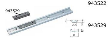
guide rails 200mm with widthness 20mm aluminium anodised profile, highness 8,2mm highness 8,2mm, max. loading 15 Kg/Pr (vertical) (delivery on request; also possible 400/800mm)
