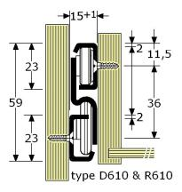
easy mounting: all 15mm single for 50 Kg (9125..) single for 100 kg (9150..) full extension for 50 Kg (9261..)
