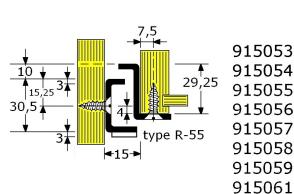
single extension drawer slide (2-parts) stainless steel 1.4509/A2 (new @) single extension 75%, heavy duty space required 15mm, for bottom mounting with stainless steel ball bearing rollers (2x ø24mm, 2x ø28mm) cabinet profile and drawer profile with screwholes 4,5mm; for easily disconnecting every day by lifting-up the front of the opened drawer; stainless steel endstop; slide can be used for -25°C. till +80°C.
