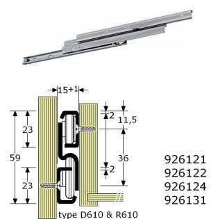
full extension drawer slide (3-parts) stainless steel 1.4509/A2 (new stainless steel @) full extension +45mm (for 30cm: +20cm), progressive action space required 15mm, highness 59mm, side mounting \*\*\*
