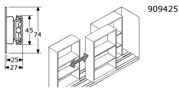
precision ball bearing slide stainless steel 304/A2 full extension, extension lengths 100% length 100cm, extension 103cm with big steel ball bearing, for 50 Kg/Pcs. width 27mm: for side mounting or high 27mm: for base mounting sales by piece (delivery on request)
