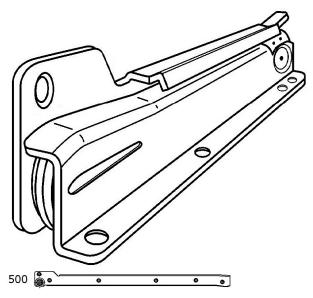
single extension drawer slide (2-parts) stainless steel 1.4509/A2 (new @) single extension 75% space required 15mm, for bottom mounting
