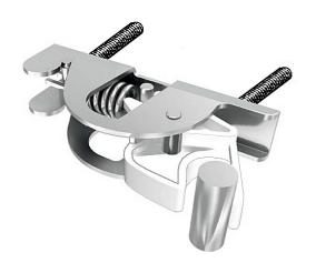
928297 drawer lock mechanism for back mounting stainless steel 304/A2 with stainless steel spring with white nylon catch for pin ø8mm or M8 (pin or pin plate not included) adjustable with 2x thread M6x40 c.t.c. 60mm without back plate, without mounting plate
