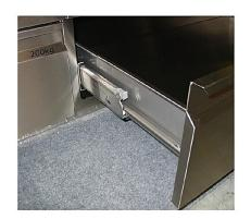
full extension drawer slide (3-parts) stainless steel 1.4509/A2 (new @) full extension -/-15mm, progressive action space required 24mm, highness 72mm for bottom mounting without screwholes
