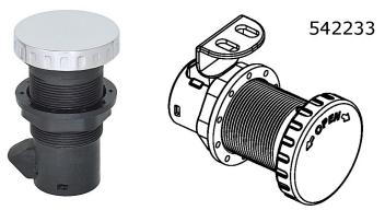
cabinet door/drawer push latch ø36mm gripped knob stainless steel 304/A2 mirror polished black nylon body with black nylon nut dead bolt will be locked when knob is pushed in open: turn ±10° the knob left or right, the knob will be coming out and
