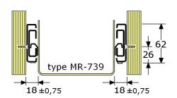
full extension drawer slide (3-parts) stainless steel 1.4509/A2 (new stainless steel @) full extension -/-15mm, progressive action space required 18mm, highness 62mm, side mounting \*\*\*
