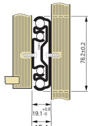
precision ball bearing slide, heavy duty steel zinc plated
