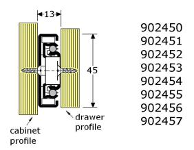
precision ball bearing slide steel zinc plated full extension slide, extension lenghts 100% space required only 13mm, highness 45mm, side mounting
