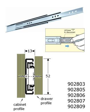
precision ball bearing slide steel zinc plated full extension slide, extension lengths 100% space required only 13mm, highness 52mm, side mounting
