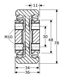
precision ball bearing slide, heavy duty steel zinc plated
