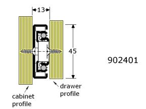
precision ball bearing slide "push-to-open" steel zinc plated full extension (3-parts), extension lengths 100% space required only 13mm, highness 45mm, side may
