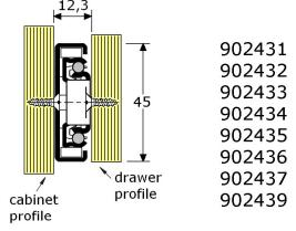
precision ball bearing slide steel zinc plated full extension slide
