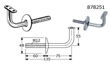
handrail bracket with flat fixing plate 15mm stainless steel 304/A2 satin polished distance wall - centre 50-75mm material/support ø12mm unvisable mounting, with threaded bolt M12x60 with self-clamping rose ø48mm (without screwholes) in boxes of 100 Pcs. (delivery on request)
