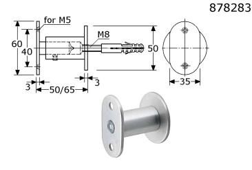
handrail bracket for side mounting stainless steel 304/A2 satin polished adjustable distance 50-65mm base/body ø25mm oval rose 50x35mm with 2 countersunked holes wall rose ø50x3mm with hole M8 in boxes of 10 Pcs. (delivery on request)
