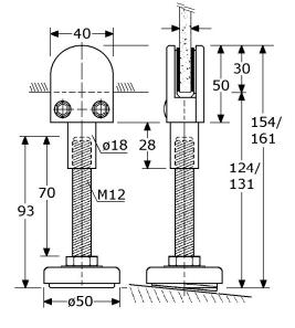
PIROSTA floor panel holder, adjustable M12 stainless steel 304/A2 satin polished flexible foot complete stainless steel 304/A2 ø50mm total high 154/161mm, opening 124/131mm ### modern design, complete stainless steel ### rounded clamp 50x45mm for 6-10mm glass/plate with black rubber packing for 6-8-10mm glass standard useful for maximum 12mm TRESPA-plate in boxes of 10 Pcs.
