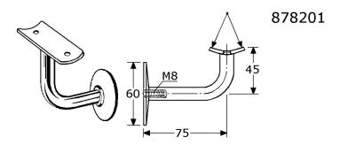
handrail bracket for tube ø40-50mm stainless steel 304/A2 satin polished distance wall - centre 75mm material/support ø12mm unvisable mounting, backside with hole M8 with wall rose ø60mm without screwholes in boxes of 100 Pcs. (delivery on request)
