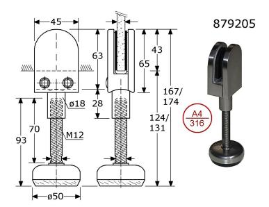
PIROSTA floor panel holder, adjustable M12 stainless steel 316/A4 polished foot stainless steel 316/A4 ø50mm with black rubber total high 167/174mm, opening 124/131mm ### modern design, totally S.S.-316/A4 ### rounded clamp 65x45mm for 6-10mm glass/plate with black rubber packing for 6-8-10mm glass standard useful for maximum 13mm TRESPA-plate in boxes of 10 Pcs.
