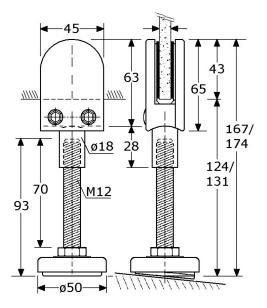
879215 PIROSTA floor panel holder, adjustable M12 stainless steel 304/A2 satin polished flexible foot complete stainless steel 304/A2 ø50mm total high 167/174mm, opening 124/131mm ### modern design, complete stainless steel ### rounded clamp 65x45mm for 6-10mm glass/plate with black rubber packing for 6-8-10mm glass standard useful for maximum 13mm TRESPA-plate
