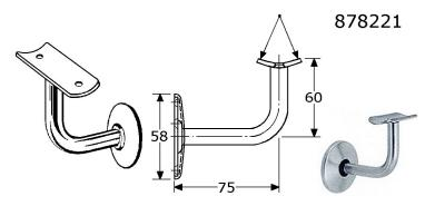
handrail bracket for tube ø40-50mm stainless steel 304/A2 satin polished distance wall - centre 75mm material/support ø12mm unvisable mounting with self-clamping rose ø58mm rose ø55mm with 3 countersunked holes (4,5/5mm) in boxes of 12 Pcs.
