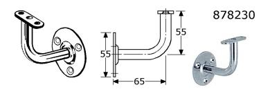
handrail bracket with flat fixing plate 15mm stainless steel 304/A2 satin polished distance wall - centre 65mm material/support ø12mm rose ø55mm with 3 countersunked holes (4,5/5mm) in boxes of 12 Pcs.
