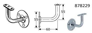
handrail bracket with flat fixing plate 15mm stainless steel 304/A2 mirror polished distance wall - centre 60mm material/support ø12mm rose ø55mm with 3 countersunked holes (4,5/5mm) in boxes of 12 Pcs.
