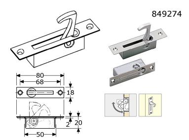
flush lift edge pull 80x18mm stainless steel 304/A2 satin polished with falling stainless steel hook fully flat front plate 80x18x2mm, rectangular with closed stainless steel case 50x15mm bore opening 50x15mm, bore depth 2+18=20mm with 2 countersunked screwholes (3,5/M4) in boxes of 20 Pcs.
