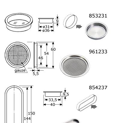
flush pull ø36mm stainless steel 304/A2 satin polished complete stainless steel, out of 1 piece bore opening ø31mm, bore depth 9mm in side-wall are 2x little nail holes in boxes of 25 Pcs.
