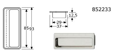
flush pull 93x37mm stainless steel 304/A2 satin polished flat stainless steel frontplate + stainless steel body bore opening 85x29mm, bore depth 1,5+12,5mm integrated single lipped, hand opening 82x18mm no screwholes, unvisable mounting in side-wall are 2x little nail holes ø1mm in boxes of 25 Pcs.
