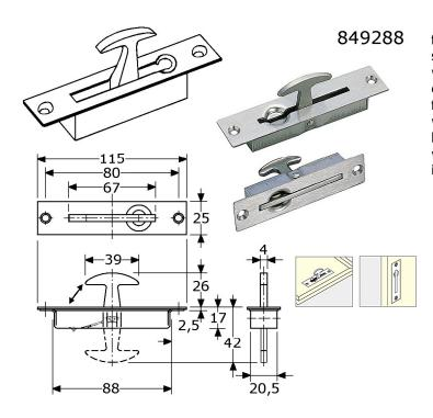
flush lift edge pull 115x25mm stainless steel 304/A2 satin polished with falling stainless steel "T"-ring open position: "T"-ring wanted to stay by spring fully flat front plate 115x25x2,5mm, rectangular with closed stainless steel case 88x20,5mm bore opening 88x20,5mm, bore depth 42mm with 2 countersunked screwholes (3,5/M4) in boxes of 20 Pcs.
