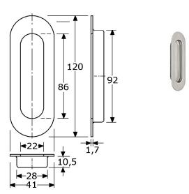
flush pull 120x41mm, rounded stainless steel 304/A2 satin polished complete stainless steel, welded body bore opening 92x28mm till 94x30mm bore depth 1,7+10,5mm integrated double lipped, hand opening 86x22mm no screwholes
