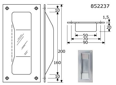
flush pull 200x90mm stainless steel 304/A2 satin polished complete stainless steel, out of 1 piece bore opening 160x50mm, bore depth 1,5+20mm integrated single lipped, heavy duty with 4 countersunked screwholes (3mm/M3) in boxes of 10 Pcs.
