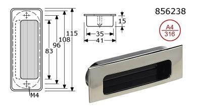
flush pull 115x41mm stainless steel 316/A4 mirror polished flat stainless steel front plate, thickness 3-4mm with black PVC body 108x35mm bore opening 108x35mm, bore depth 15mm unvisable mounting: backside with 2x hole M4 c.t.c. 96mm
