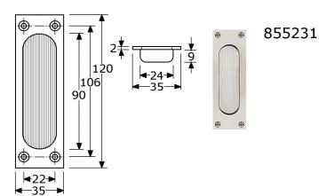
flush pull 120x35mm stainless steel 304/A2 satin polished complete stainless steel, welded body bore opening 90x24mm, bore depth 2+9mm with 4 countersunked screwholes (screws M4x7) in boxes of 25 Pcs.
