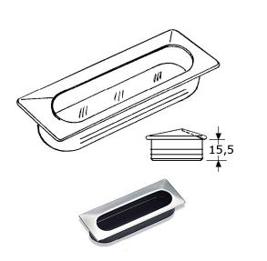
856214 flush pull 75x36mm stainless steel 304/A2 satin polished modern stainless steel front plate highness 7mm with black PVC body 71x30mm bore opening 71x30mm, bore depth 15,5mm in boxes of 40 Pcs.
