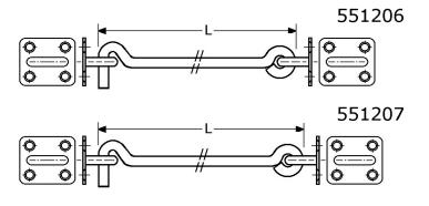
gate hooks, length L=160x5,2mm stainless steel 304/A2 with 1 loose & 1 fixed eye plate 35x30x3mm with each 4 countersunked screwholes (3,5/4mm/M4) packed in boxes of 10 Pcs.
