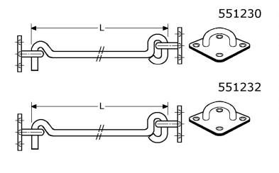
gate hooks, length L=300x6,0mm stainless steel 304/A2, with long eyes with 1 loose & 1 fixed diamond plate 80x50x5mm with each 4 countersunked screwholes (6mm/M6) packed in boxes of 10 Pcs.
