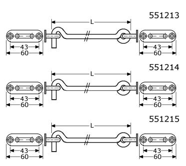
gate hooks, length L=120x4,4mm stainless steel 304/A2 with 1 loose & 1 fixed eye plate 60x20x2,5mm handy long narrow version, eye thickness ø6mm with each 2 countersunked screwholes (4/4,5mm) packed in boxes of 10 Pcs. (delivery on request)
