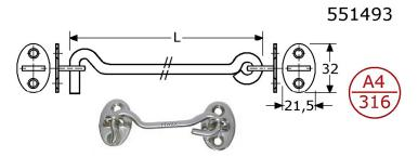
gate hooks, length L=100x4,4mm stainless steel 316/A4 mirror polished with 1 loose & 1 fixed eye plate 32x21,5mm with each 2 countersunked screwholes (4mm) in boxes of 10 Pcs.
