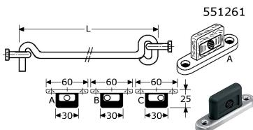
gate hooks, length L=500x6,0mm stainless steel 304/A2, with long eyes with 1 loose & 1 fixed black rubber plate 60x16mm with each 2 countersunked screwholes stainless steel cover, highness 25mm, hole ø7mm hole in the centre (=A) or left (=B) or right (=C) packed in boxes of 10 Pcs. (delivery on request)
