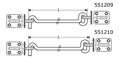
gate hooks, length L=300x6,0mm stainless steel 304/A2, with long eyes with 1 loose & 1 fixed eye plate 40x35x3mm with each 4 countersunked screwholes (4,0/4,5/M5) packed in boxes of 10 Pcs.
